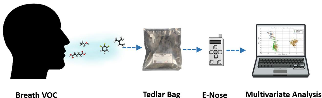
Fig. 1 Schematic of the experimental procedure for breath VOC analysis
